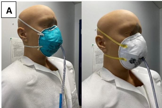
Fig. 2A. Medium Static Advanced Headform. 3M 1860 (Left), 3M 8210 (Right)
