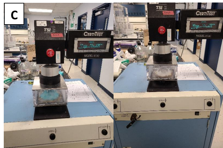
Fig. 2C. TSI 8130 Filter Tester 3M 1860 (Left), 3M 8210 (Right)
