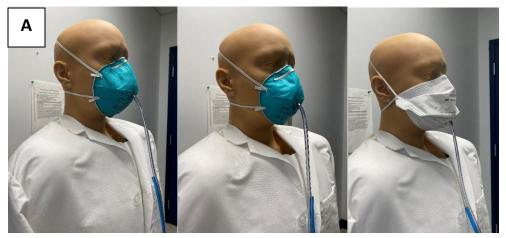
Fig. 2A. Medium Static Advanced Headform (left to right: 3M 1860, 3M 1860S, VFlex 1804)
