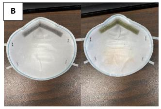
Fig. 1B. 3M 1860 Inside Control (Left), Treated (Right)
