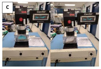
Fig. 2C. TSI 8130 Filter Tester (left to right: 3M 1860, VFlex 1804)
