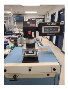
Figure 2. Laboratory Test Photo (TSI, Inc. 8130 filter tester). Due to the design of this respirator, the filter housing was removed from the device and tested for filtration.
