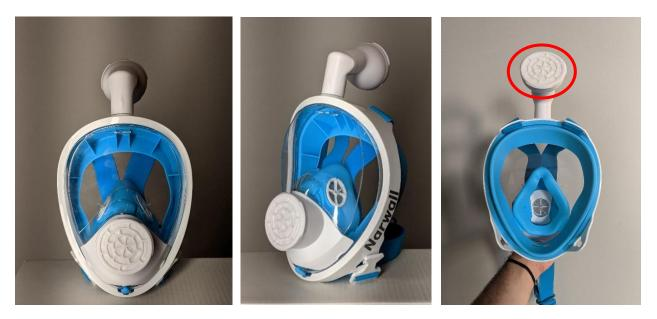
Figure 1: Narwall Mask LLC front (left image), side (middle image) and interior (right image) views. The filter is shown in the red circle and was removed for filtration testing.
