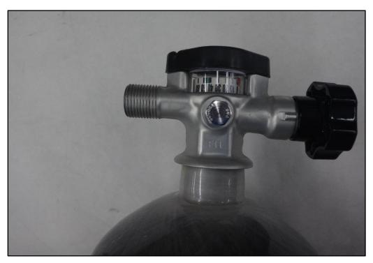
Figure 30: Cylinder gauge and threads.
