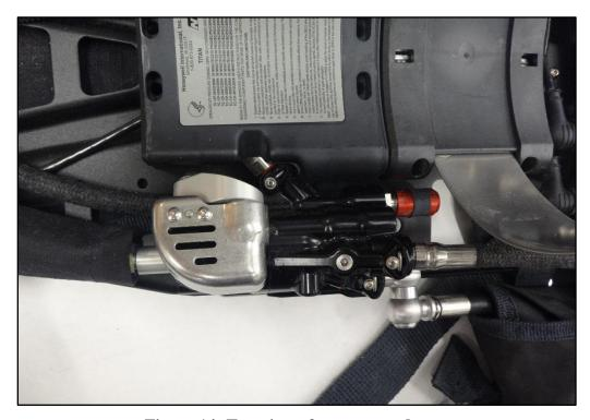
Figure 14: Top view of pressure reducer.
