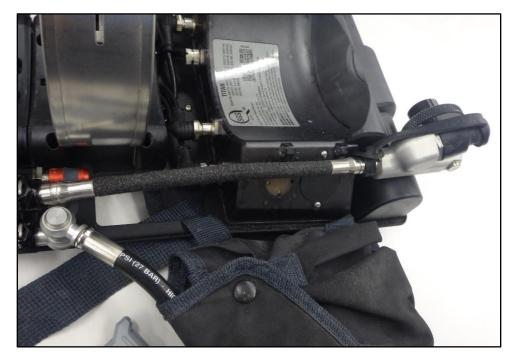
Figure 16: High pressure line.
