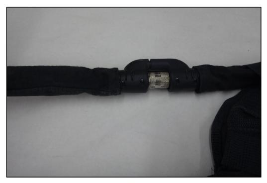
Figure 12: Quick Disconnect on low pressure line.
