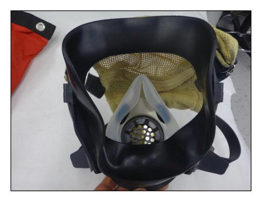
Figure 6: Inside view of facepiece, skirt, and nosecup.
