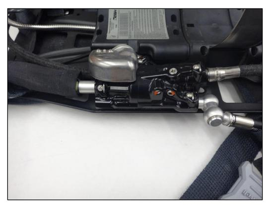
Figure 13: Pressure reducer assembly.
