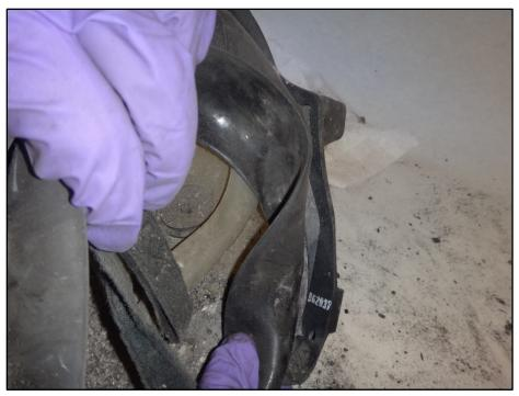
Figure 7: Identifying markings on facepiece frame
