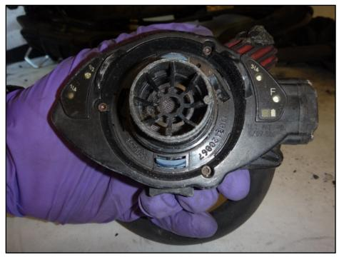
Figure 10: Inside flange, mask mounted regulator
