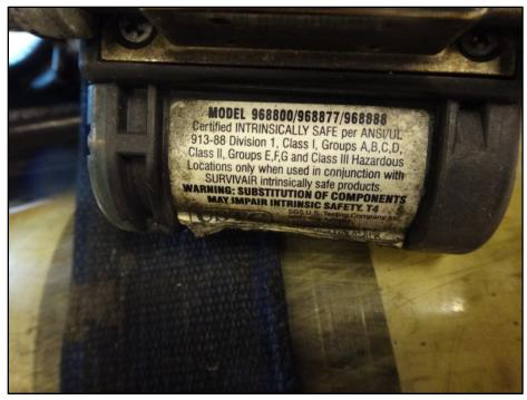
Figure 14: Identifying markings on pressure reducer
