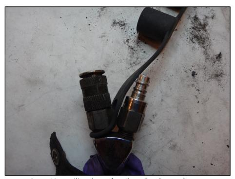
Figure 28: Auxiliary hose, female and male attachments
