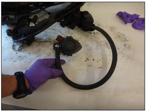
Figure 9: Mask mounted regulator
