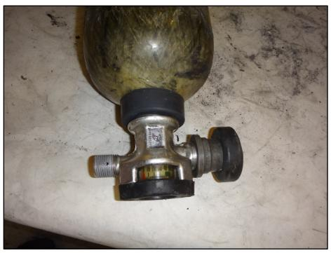
Figure 27: Cylinder threads with readable cylinder gauge
