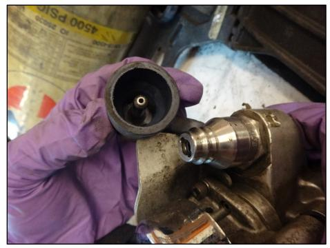
Figure 18: Quick fill port on cylinder attachment
