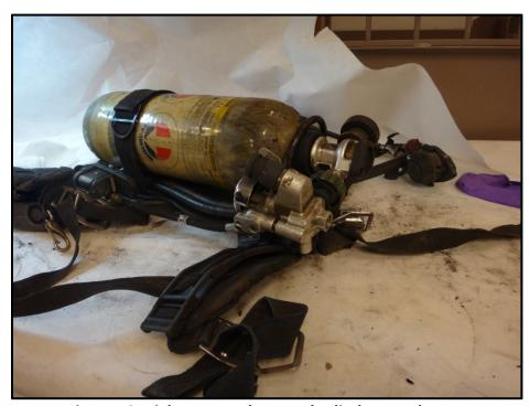
Figure 16: High pressure hose and cylinder attachment
