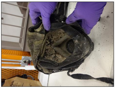
Figure 5: View of inside of facepiece, covered in debris
