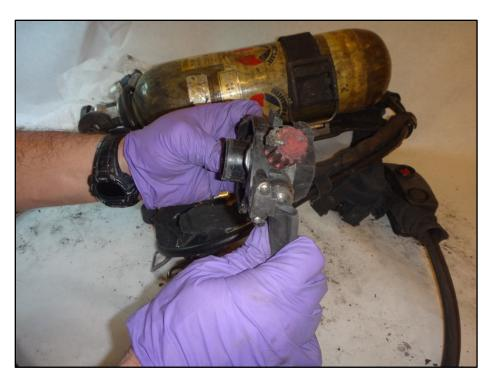
Figure 11: Heat damage to air supply valve
