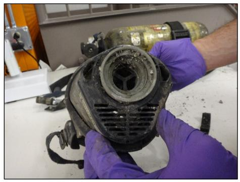
Figure 6: Bottom view of facepiece, debris inside
